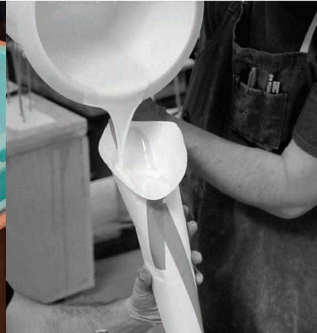
Air bubbles are removed with a vacuum chamber and the resin is poured by hand.
